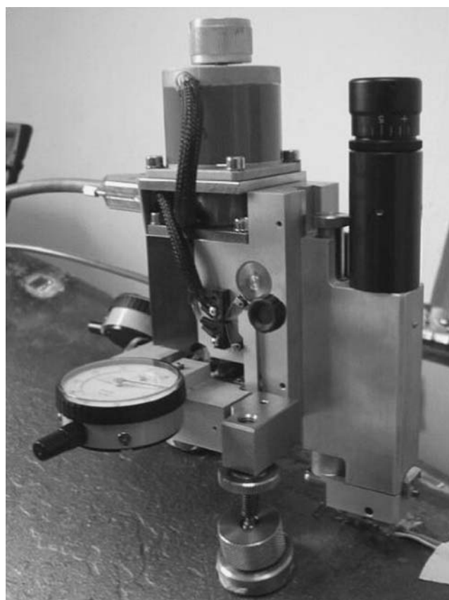
Fig. 7 Hole drilling RESTAN apparatus: An optical microscope is mounted coaxially to the end mill, and a centesimal dial gauge serves for the measurement of hole eccentricity.
